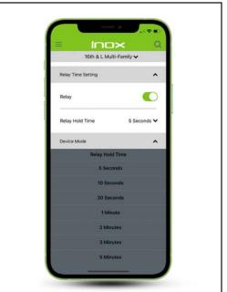
The default timing on the closing circuits is 5 seconds. In the Smart Mode, this timing is adjustable from 5 seconds to 5 minutes using the Smart APP in Device Settings.
