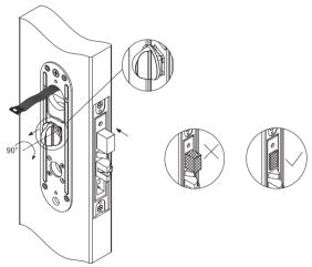
After aligning thumbturn spindle with sub-plate, slightly pull alignment tool from square cut-out enough so that it can be turned 90° to test deadbolt operation.
